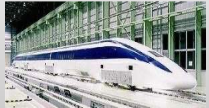
The Yamanashi MLX01 MagLev test vehicle achieved a speed of 343 mph (552 kph) on April 14, 1999
